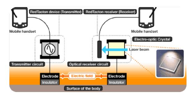
The naturally occurring electric field induced on the surface of the human body dissipates into the earth. Therefore, this electric field is exceptionally faint and unstable. The photonic electric field sensor developed by NTT enables weak electric fields to be measured by detecting changes in the optical properties of an electro optic crystal with a laser beam.
